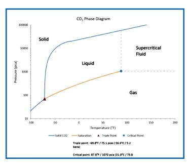
CO2 remains as a liquid in the storage vessel, meaning the temperature and pressure must remain above the triple point of -69.8°F and 75.1 psia (~60 psig) and below the critical point of 87.8°F and 1070 psia (1055 psig)
