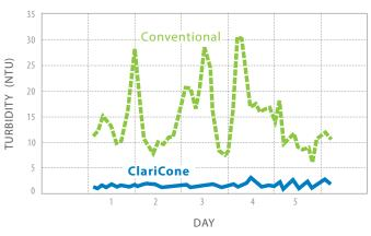
The ClariCone system's superior performance compared with conventional solids contact clarifiers is illustrated by operating data from side-by-side clarifiers.
