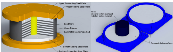
Figure 4. Seismic isolators – lead-rubber isolator (left) and friction pendulum isolator (right).
