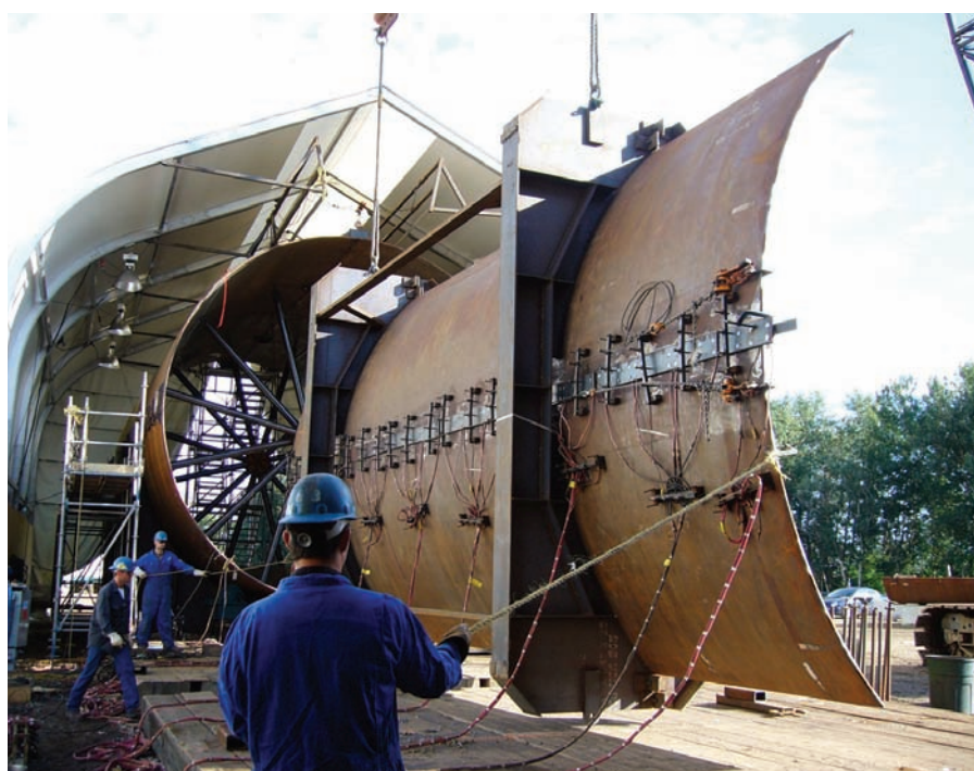
Fig. 4 — Preheat applied by electric resistance heaters formed to fit the vessel shell.
