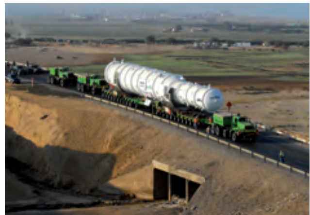
Significant modifications were required to the Pan American highway to enable the transfer of the equipment to the site, in particular for two of the larger and heavier pieces of equipment, such as the MCHC (pictured)
