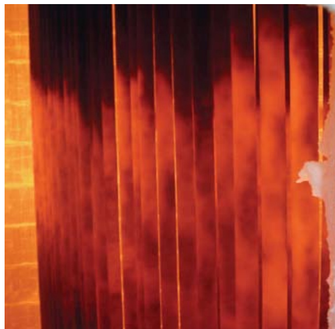
FIG. 3 Reformer tubes exhibiting the possible effects of carbon formation, sulfur poisoning, catalyst deactivation and/or catalyst attrition.
