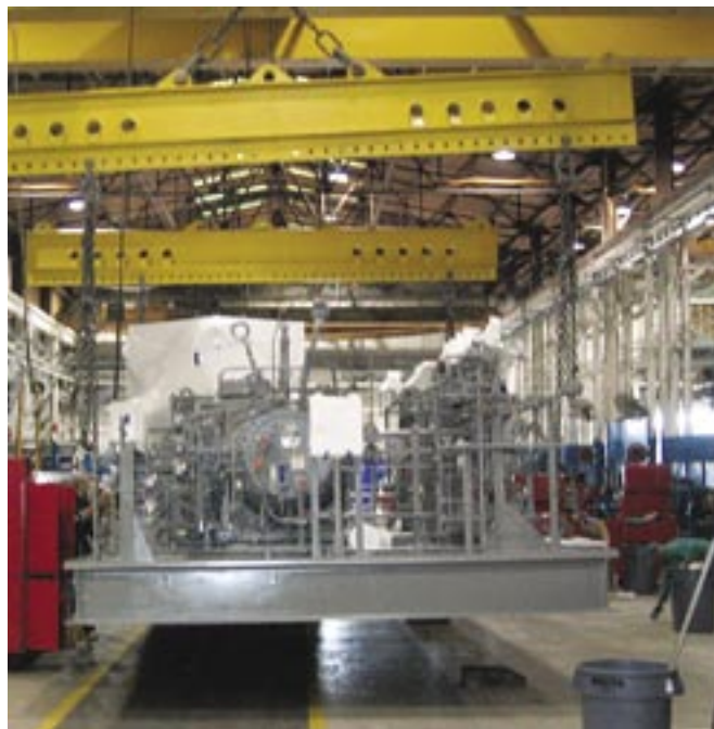
FIG. 3 Fabricated equipment in the shop is mounted onto a skid, which is then transported to the site.
